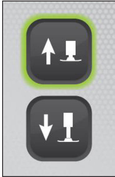
Outrigger Extend / Retract switch
