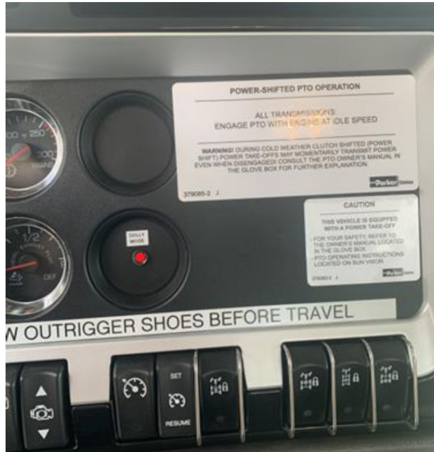
Carrier Cab Dolly Transport Indicator Lights
