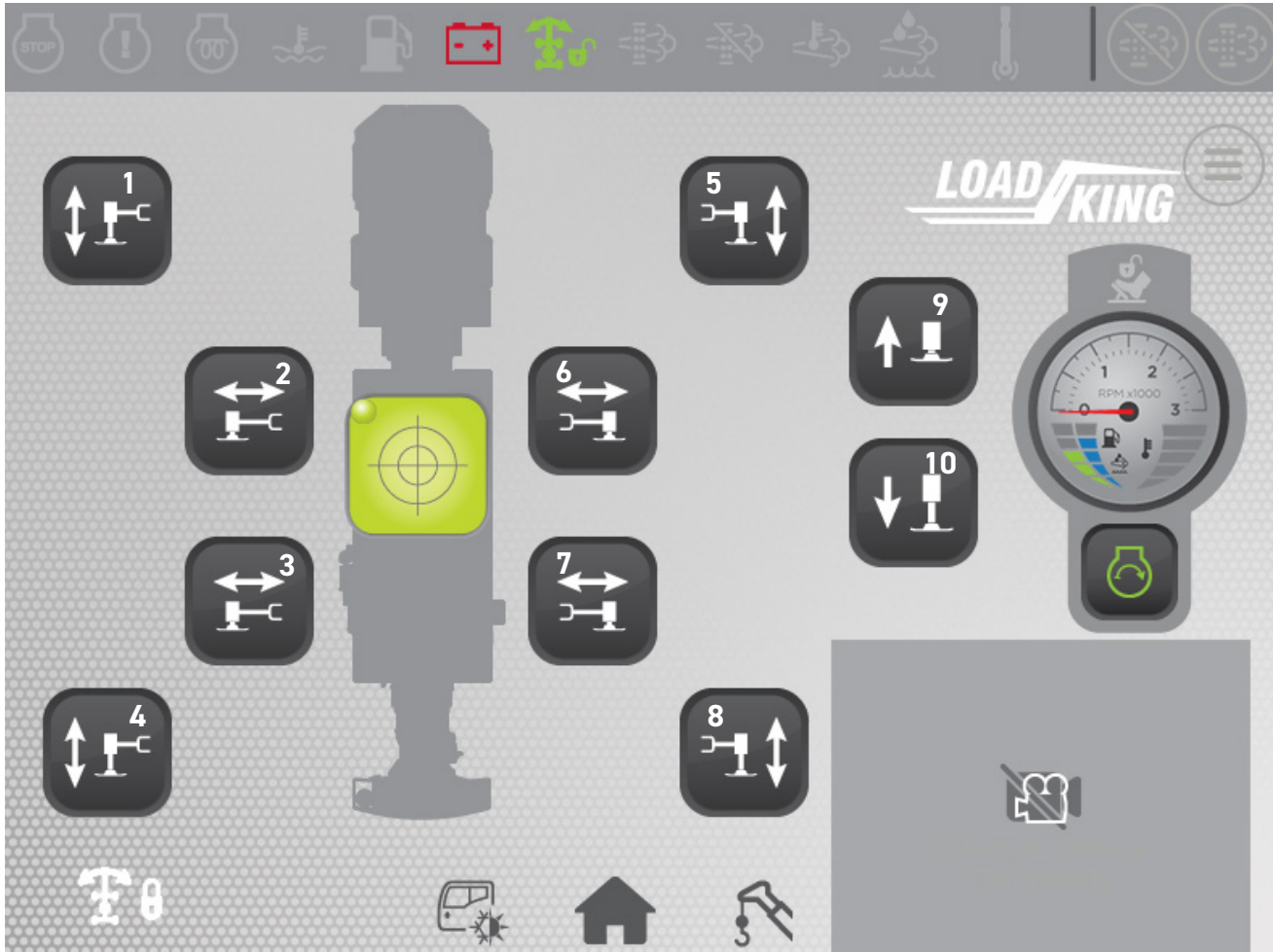
Outrigger Controls Screen
