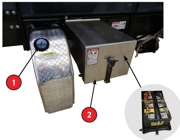
Battery Box Location - Under Left Side of Vehicle
