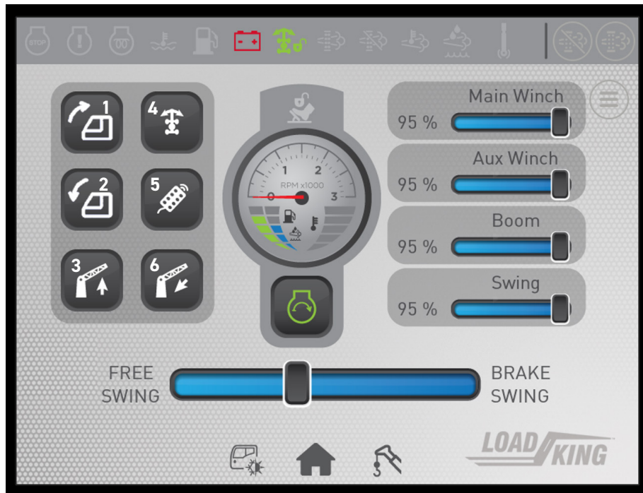
Lifting Control Screen
