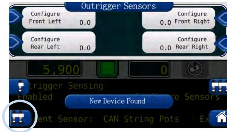
7. Move the outriggers to fully extended position and press the corresponding button to set the fully extended outrigger position.
