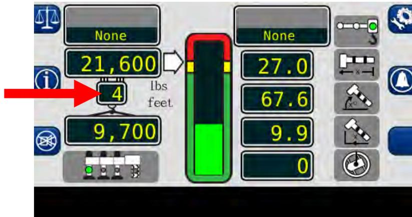
5. The **INFORMATION** button displays system generated messages regarding the software versions of the equipment and fault codes. Press and hold the **INFORMATION** button to display the data. The messages will remain on the screen until the button is released.
