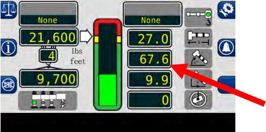
15. The **LOAD RADIUS** window displays the radius of the main boom.
