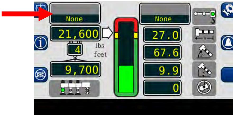
8. The **SYSTEM** has the capability of showing metric or imperial units. This can be changed in the calibration menu.
