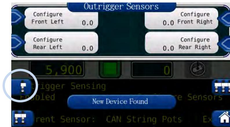
6. Move the outriggers to intermediate position and press the corresponding button to set the intermediate outrigger position.
