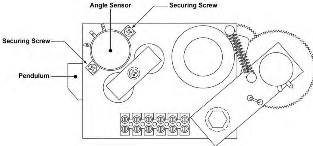
1. Place the boom at 0.0 degrees. Verify using a digital level.
