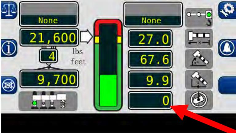
17. The **BAR GRAPH** indicates the actual load as a percent of the rated capacity of the current configuration of the machine.
