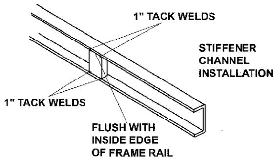
Frame stiffeners must be of the following dimensions, and be cut to length to fit snugly into the trucks frame rails.
