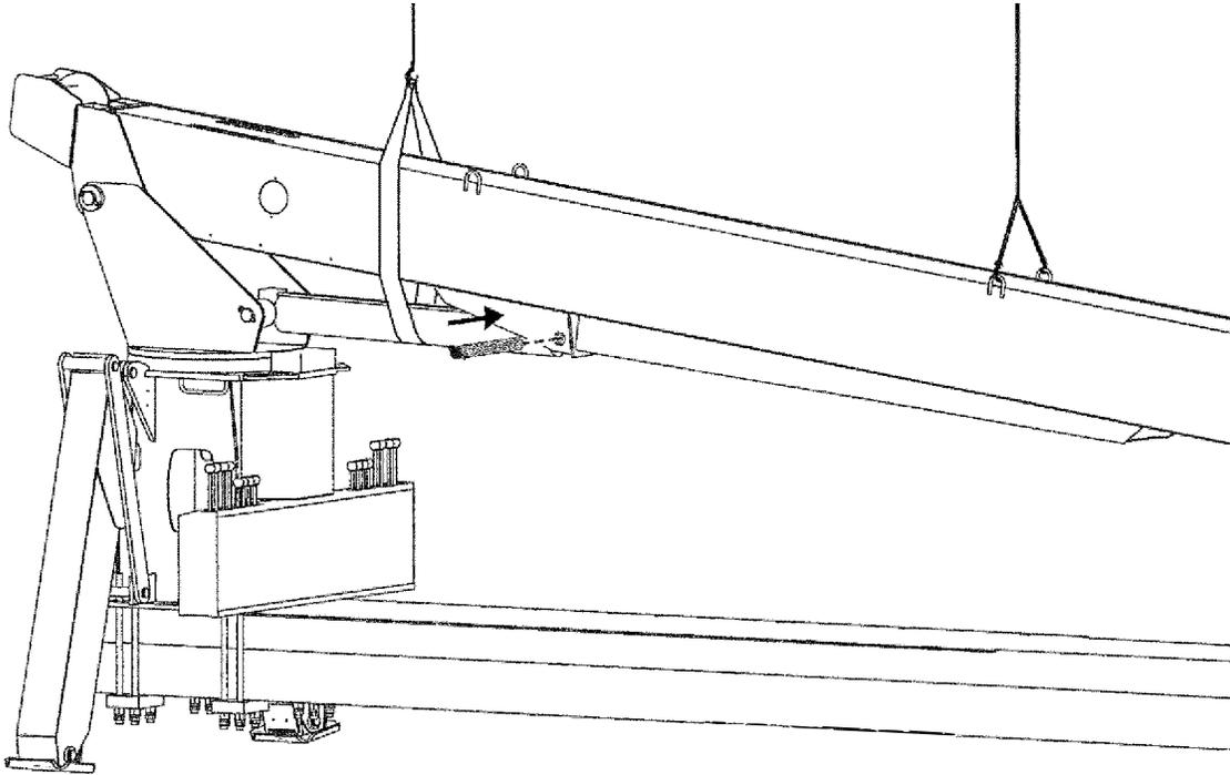
7. The hoses for the boom functions should be routed as in the Hydraulic Piping drawings.
