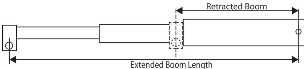
$$\text{Extended Length} - \text{Retracted Length} = \text{Span}$$
