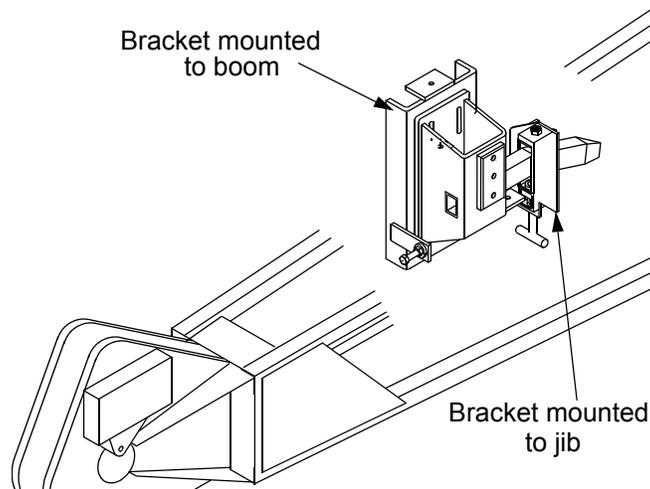
14. As the boom is retracted, verify that the stowage bracket mounted to the jib is engaging properly with the stowage bracket mounted to the boom.
