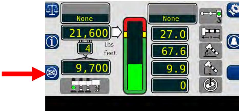
4. The **PARTS OF LINE** window displays the amount of line chosen for the configuration selected. It is adjustable from the configuration screen.
