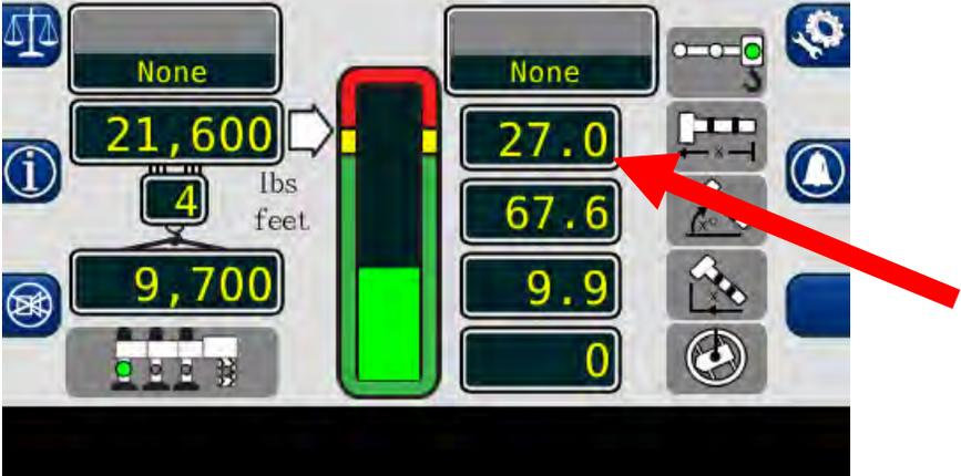
14. The **BOOM ANGLE** window displays the angle of the main boom in degrees relative to horizontal.
