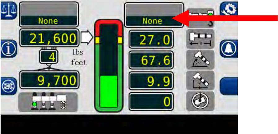
11. The **PICK POINT** icon displays the currently selected pick point chosen on the Configuration screen.
