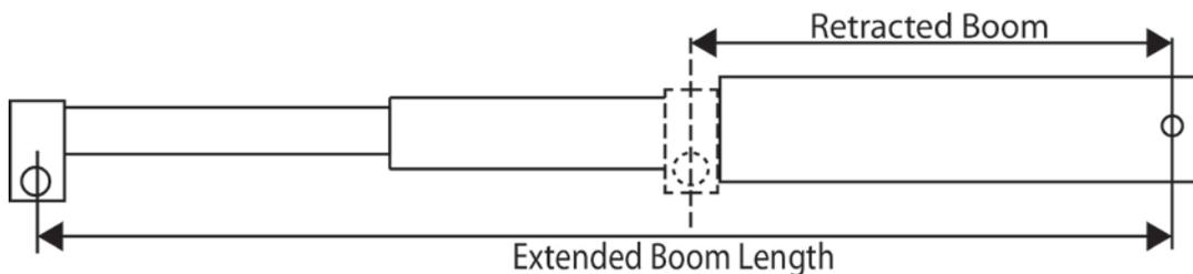
$$\text{Extended Length} - \text{Retracted Length} = \text{Span}$$
