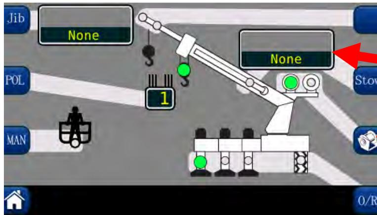
8. The **OUTRIGGER/TIRE** selections are made by pressing the **O/R** button. **NOTE:** *Some cranes will not have the option of selecting different outrigger positions.*
