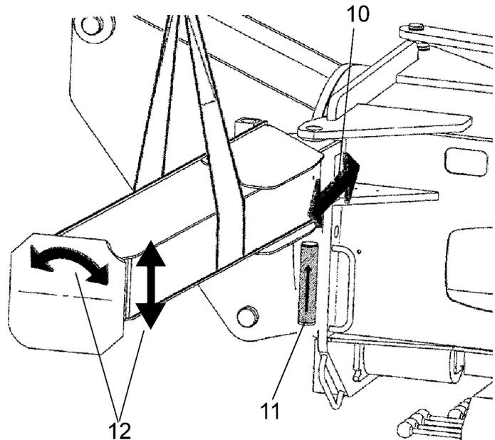
13. Once the pin is fully inserted and the snap ring groove is clear of the hole, the hoist can be lowered in order to bind the pin in place, at this point reinstall the snap ring on the pivot pin.
