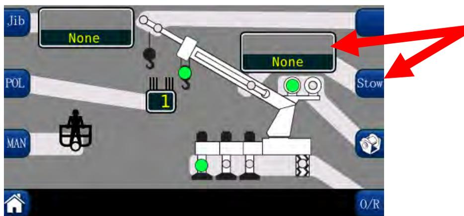
7. The **WINCH** group contains two green indicators, which indicate the selection of front or rear winch. **NOTE:** *If the crane is equipped with two winches, always select the winch to be used for the lift, prior to selecting the parts of line selections for each winch.*
