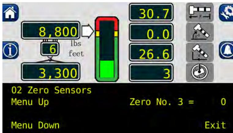
5. Press the "Zero No. 3 =" and you will be prompted with "Yes! Calibrate!" Press the button a second time to calibrate the zero. The angle sensor zero routine is complete.
