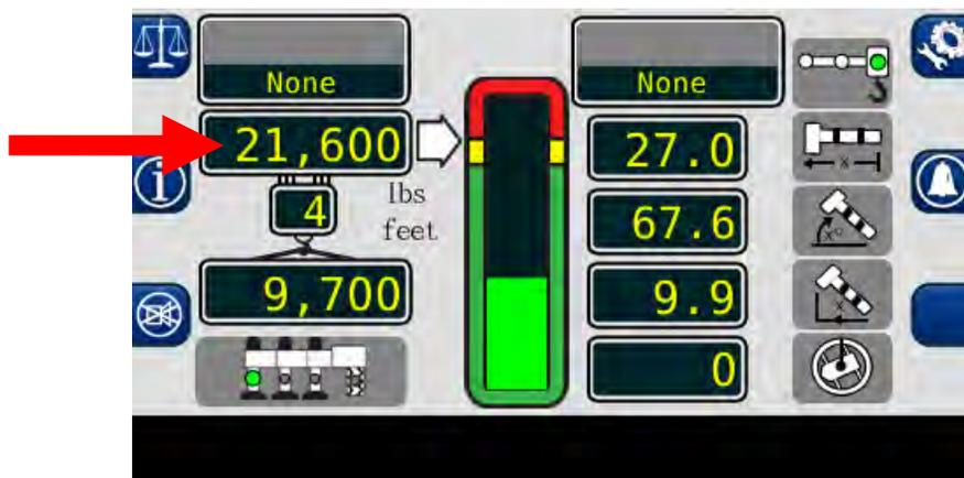
7. The **ERECTED JIB** window displays the jib option selected for the machine. If there are no jib options available, the display will show "None".
