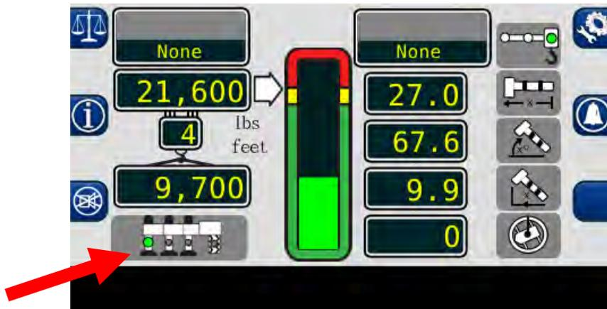
2. The **ACTUAL LOAD** value displays the total load, including slings, etc., suspended below the lifting point. **NOTE:** The system load reading is most accurate in static situations. Due to system dynamic response, the load reading may vary when lifting or lower the load. Meter functions carefully, especially boom down to minimize the dynamic effects.
