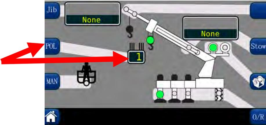
4. The **JIB OPTIONS** may be selected by pressing the **Jib** button multiple times to scroll through the jib options. If there are no options available, the display will show “None”.
