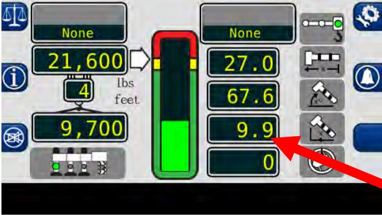
16. The **SWING ANGLE** window displays the swing of the boom relative to the zero point.
