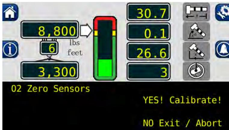
8. The display will then read “Zero No. 2 = 0”. The retracted boom length will be displayed in the boom length window. Extension sensor zero calibration is complete.
