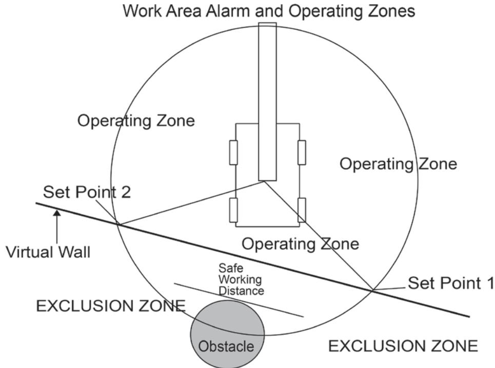
The work area alarm, defines an imaginary vertical plane between two set points. When the plane is passed the red warning indicator will be displayed, the alarm will sound, and the message “!! EXCLUSION ZONE !!” will flash as shown below.
