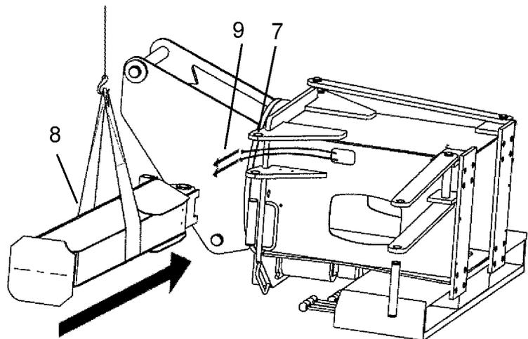
9. After removing the hydraulic caps from the top of the cylinder, immediately connect the Extend and Retract hoses to the proper ports on the outrigger cylinder. These ports should be marked with a E and R, if these are not visible, the port closest to the hydraulic piping on the side of the cylinder is the retract port.
