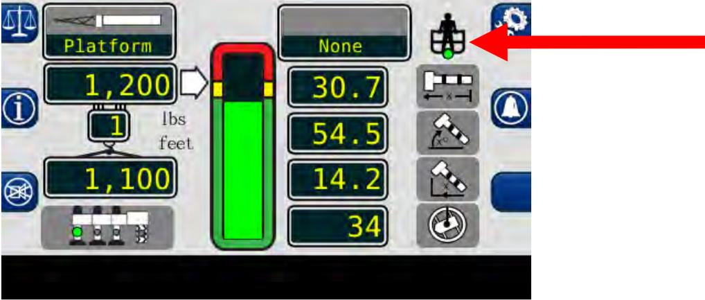
12. The **CONFIGURATION** button accesses the configuration display screen.
