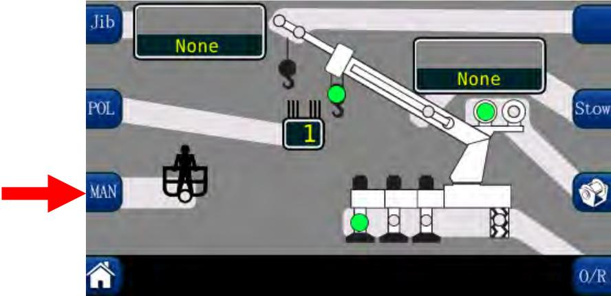
3. The **POL** button selects the current parts of line. Pressing the **POL** button will increment the parts of line. When the maximum parts of line for the equipment being used is reached, the indicator will rollover to one **POL**.
