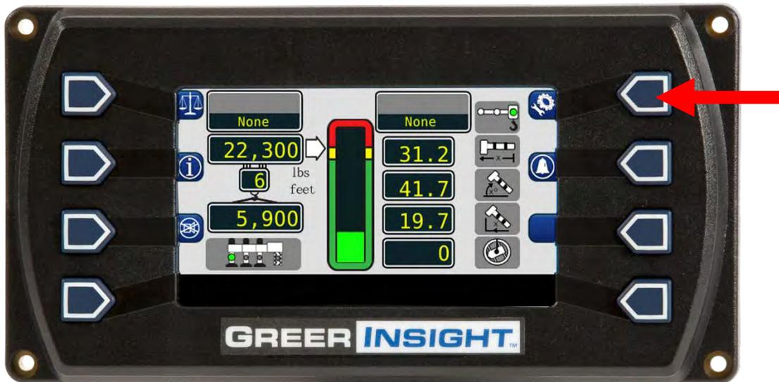
The configuration display may be accessed from the home display by pressing the **Configuration** button.
