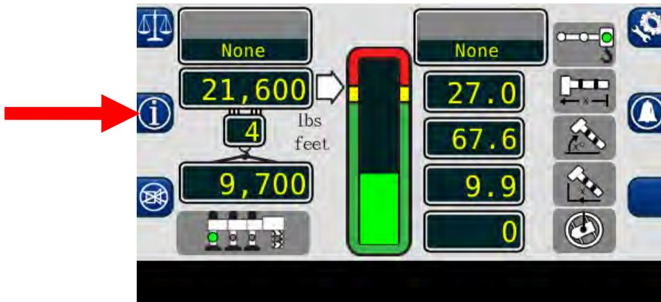
6. The **RATED CAPACITY** window displays the maximum rated capacity of the machine in the current configuration.
