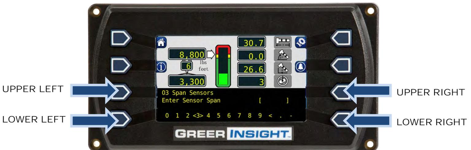
7. The lower left and lower right buttons are used to select the number. The number inside the brackets is the current selection, in the above image, the number 3 is between the brackets.
