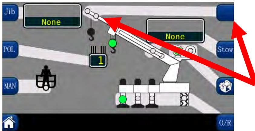
6. The **STOW (STOWED JIB)**, group contains one green indicator. This will illuminate when a jib is stowed on the boom. Press the **Stow** button multiple times to scroll through jib options. If there are no options available, the display will show “None”.
