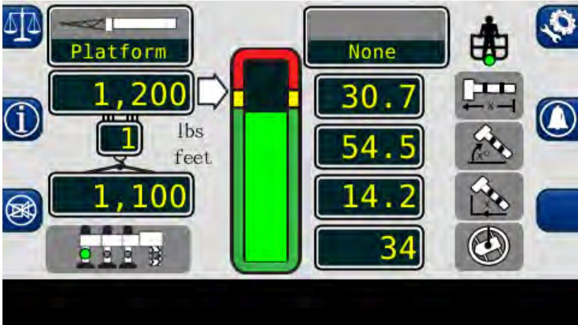
1. The **OUTRIGGER/TIRES** setting contains four green indicators. They indicate the selection of tires, full, intermediate, or retracted outriggers. The user must make the selection from the configuration display. **NOTE:** *OUTRIGGER/TIRE selections are dependent on the crane being used.*
