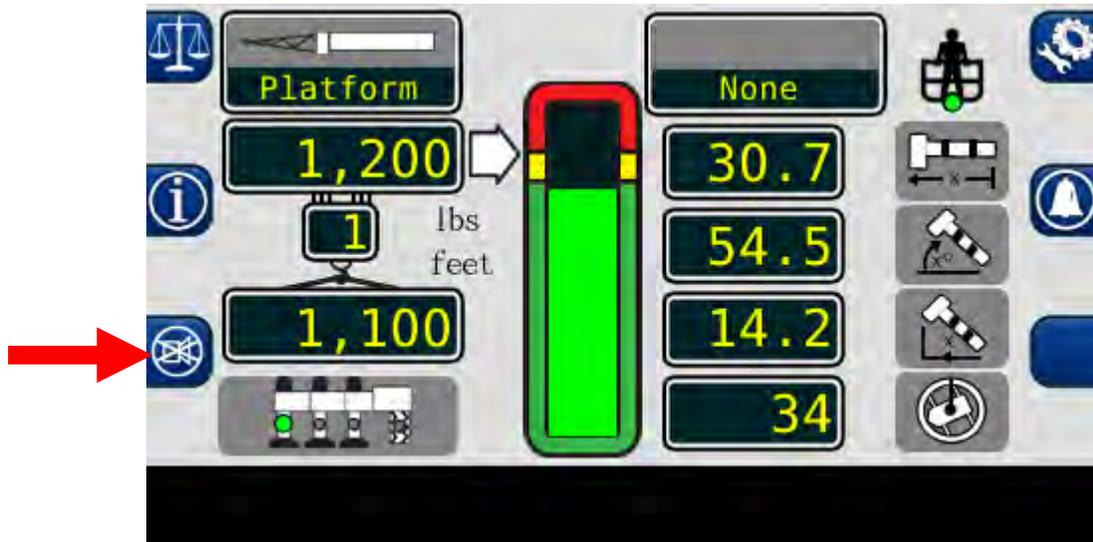
The **Cancel Alarm** button is used to silence the audible alarm. Press this button to cancel an audible alarm from an:
