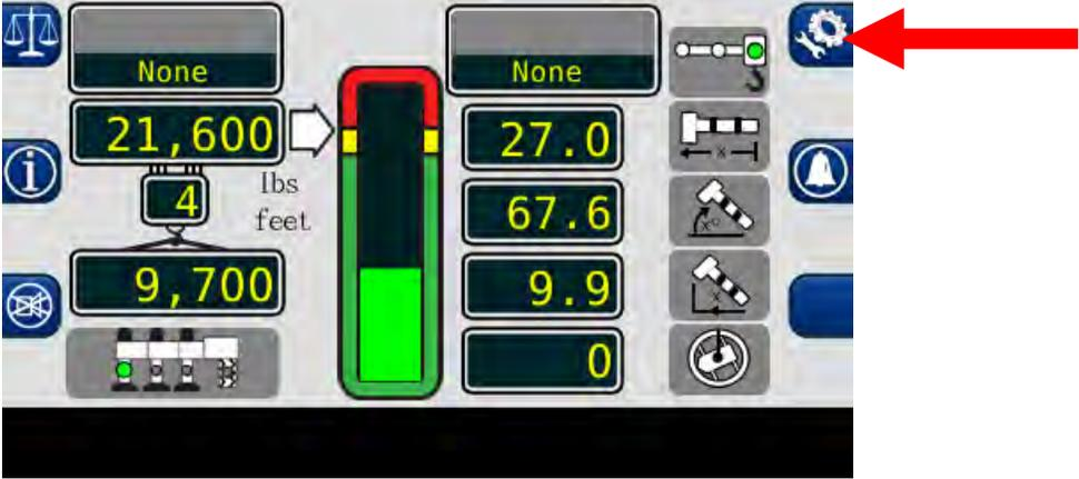
13. The **BOOM LENGTH** window displays the length of the main boom from the boom foot pin to the sheave pin of the main boom head machinery.
