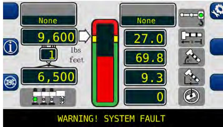
To view the fault codes, press and hold the (i) button as shown.
