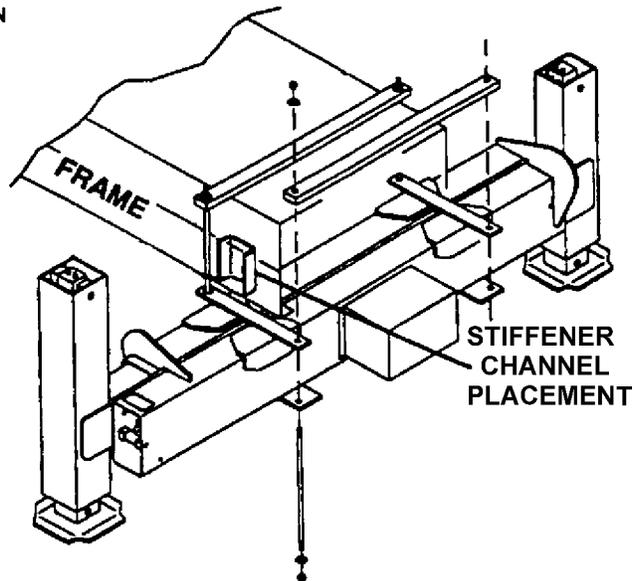
Using the subframe and flatbed as a guide, carefully layout the truck frame and determine location of the tiedown bolts for the mainframe and auxiliary outriggers. This will determine stiffener channel placement. Stiffener channel placement for auxiliary outrigger is determined by measuring 40-50 inches (1000-1270mm) from the the **rearmost axle** to the center of the auxiliary outrigger mount points.
