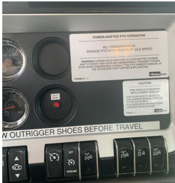
Carrier Cab Dolly Transport Indicator Lights
