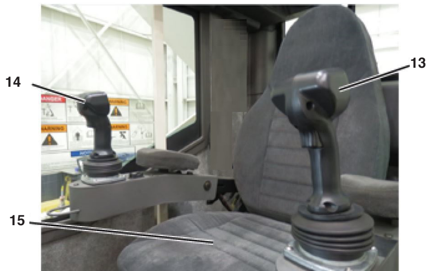
Operator's Seat Controls
