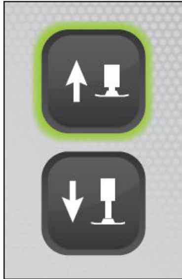
Outrigger Extend / Retract switch
