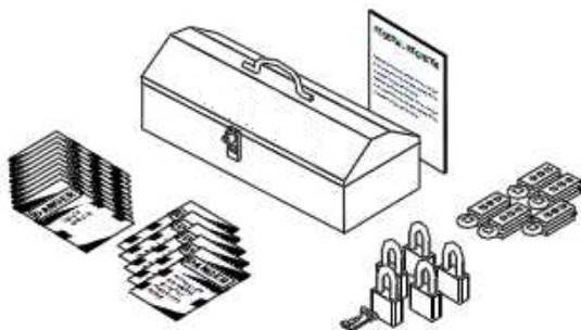
Typical Lock Out & Tag Out Kit
