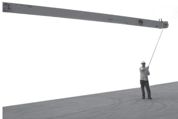
Jib controlled swing w/tag line rope - end location of rigging person
