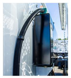
Hydraulic tank mounted on the front of the body, behind the cab, offering optimized bed and body capacity and storage
