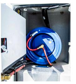
Reel-mounted air hose protected behind hinged control panel in crane compartment for maximum compartment capacity and maintenance access
