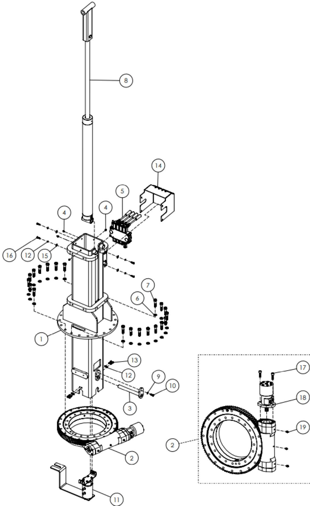
**CVR00051 SUB-ASSEMBLY, PEDESTAL ROTATION BASE/LIFT CYLINDER**
