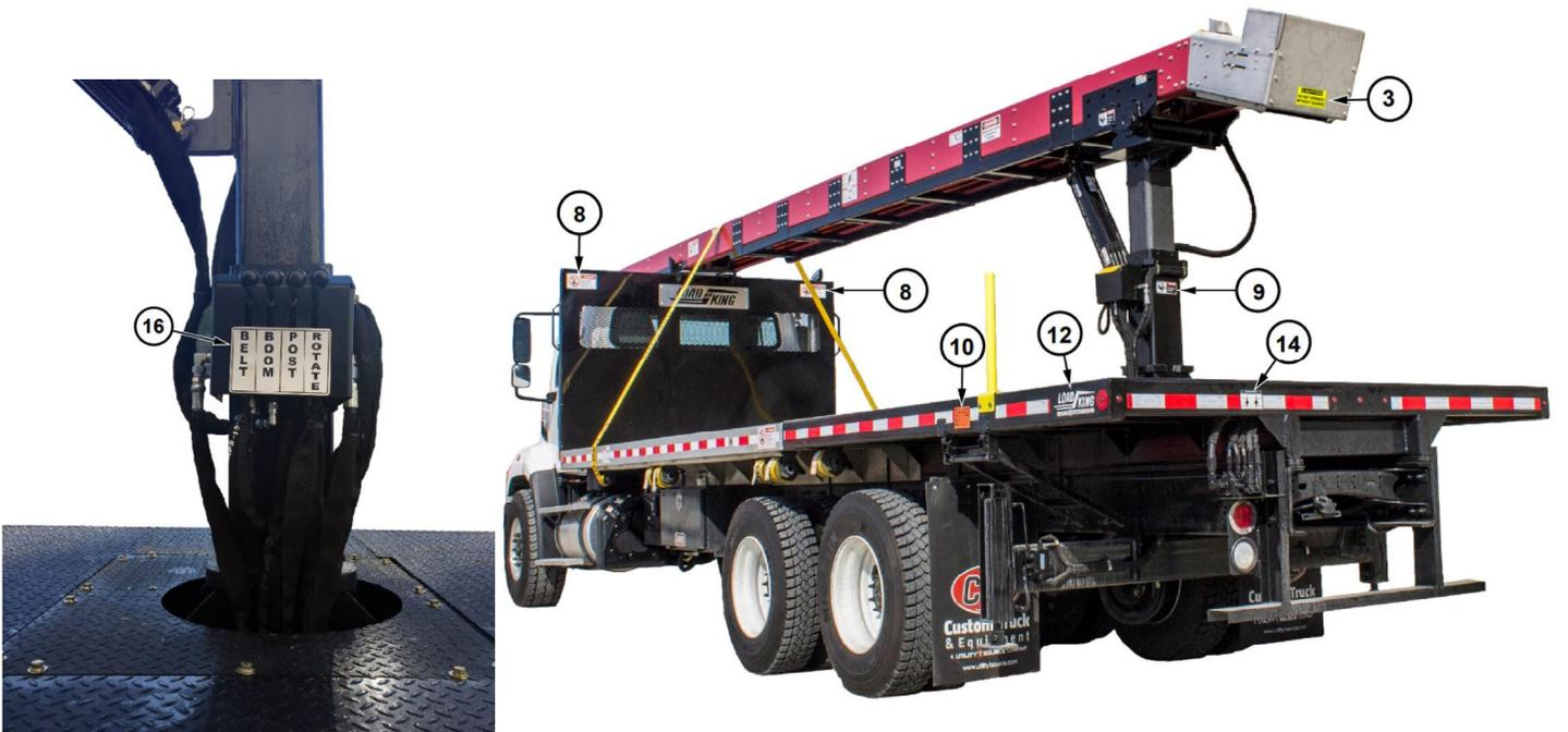
**CVR00107 ASSEMBLY, PEDESTAL W/MAST CYLINDER**
