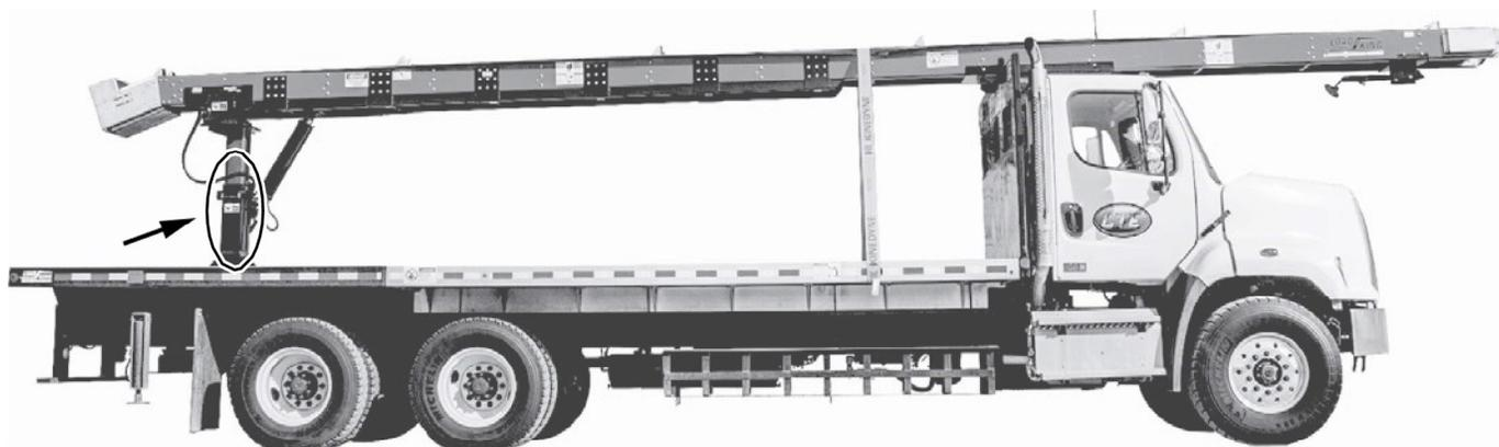
**CVR00277 ASSEMBLY, SWIVEL SHAFT UNION ROTATION PEDESTAL**
