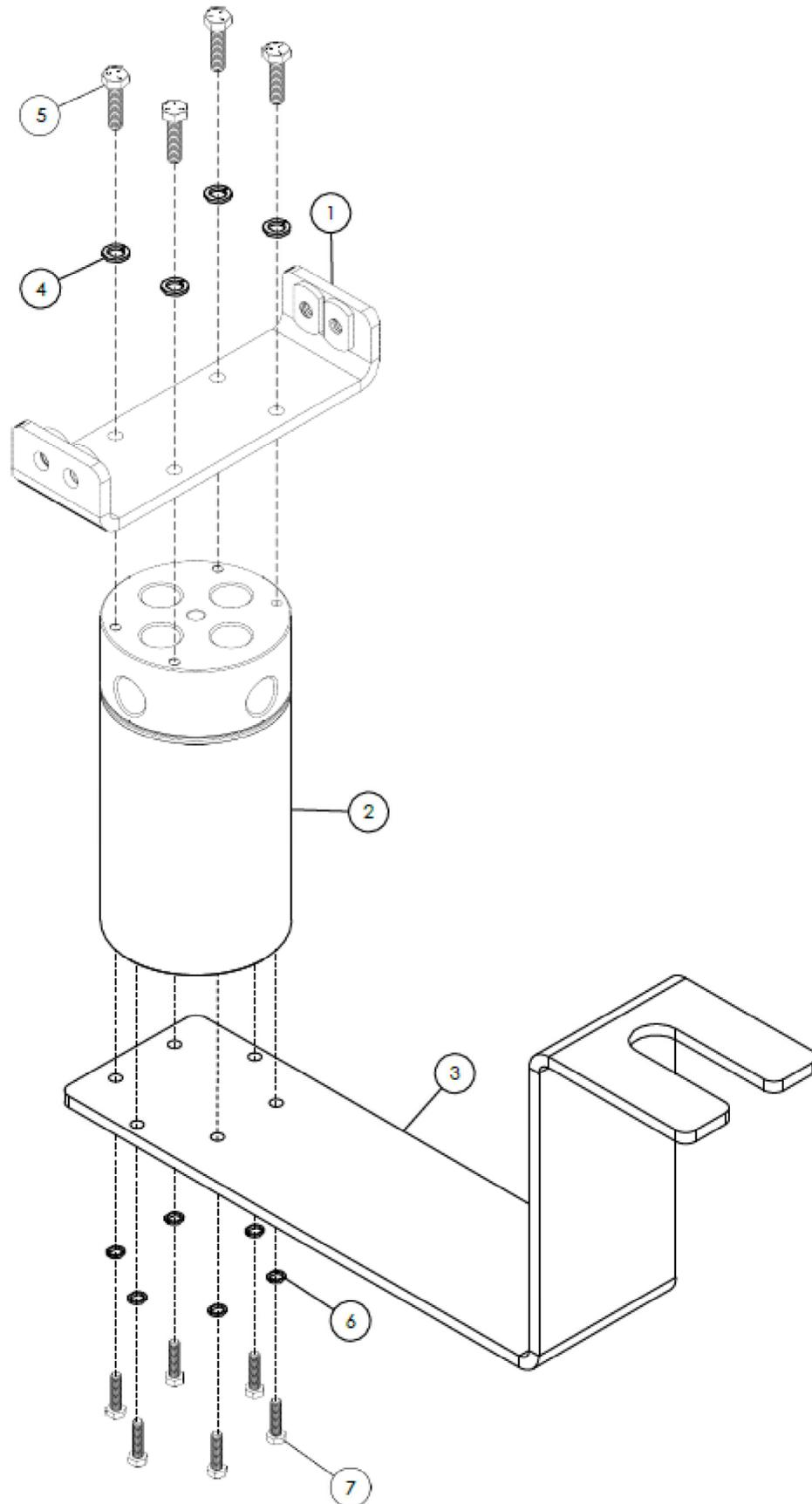
**CVR00277 ASSEMBLY, SWIVEL SHAFT UNION ROTATION PEDESTAL**
