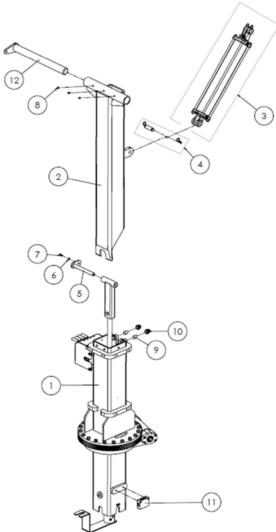
**CVR00107 ASSEMBLY, PEDESTAL W/MAST CYLINDER**
