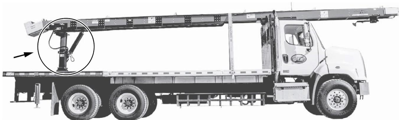
**CVR00051 SUB-ASSEMBLY, PEDESTAL ROTATION BASE/LIFT CYLINDER**
