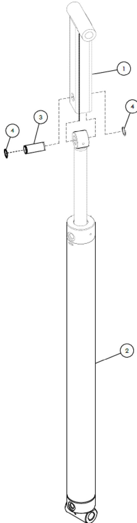
**CVR00105 ASSEMBLY, CYLINDER W/EXTENSION VERTICAL LIFT INNER PEDESTAL TOP**
